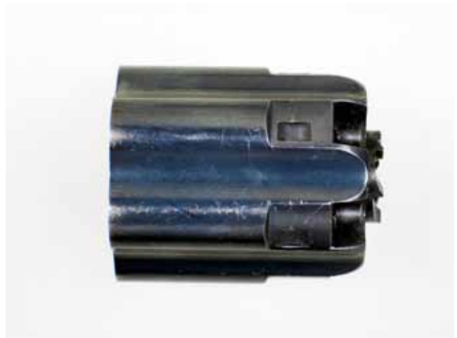
Left: While the cylinders of the no-patent pistols were drilled for safety pins, the pins, which were covered by a Colt patent, were not installed. Right: The cylinder stop slots of the no-patent pistols do not have the patented grooves leading to the slots that are on production pistols. (Paul Davis Photos. Connecticut State Museum Collection.)
