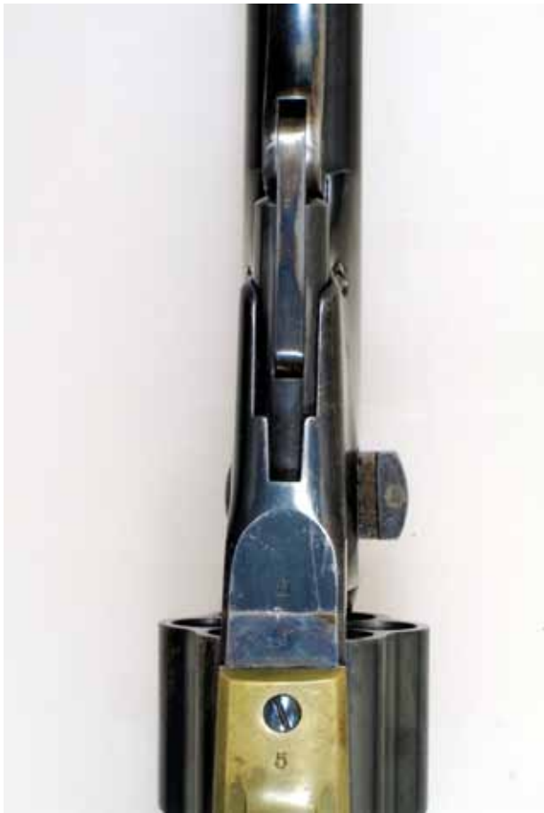
Left: Bottom view of no-patent NMA Number 5. Right, top: Note the pieced-together trigger guard on Number 5. Right, bottom: The hinged loading levers of these no-patent NMA revolvers appear to be unique to this variation. (Paul Davies Photos. Connecticut State Museum Collection)
