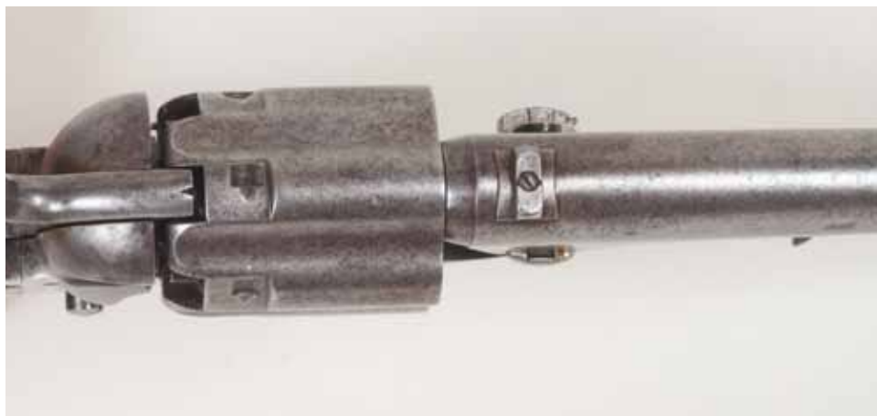
Note the odd rear sight and the absence of both barrel markings and the patented grooves leading to the cylinder stop slots. (Fred Barton Photo and Collection)
